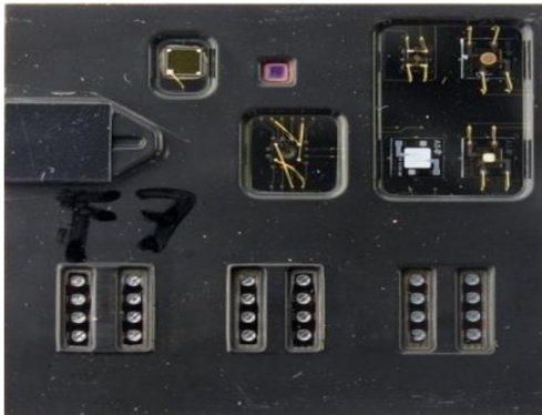
Fig.14. Over-molded 3D-integrated CMOS wafer platform including a total of 57 sensor devices.
